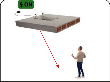
2.5 Press the opening switch of the remote to open the ladder.
