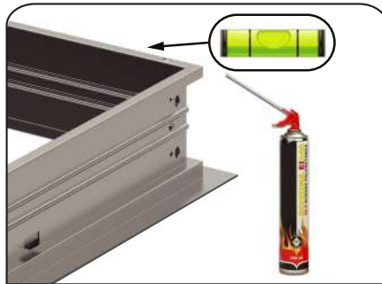
2.4 Make sure that the staircase frame is leveled! Use polyurethane foam.
